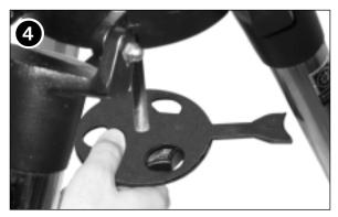
4. Remove the spreader bar (see above figure) from the shipping carton. Slide the spreader bar onto the threaded rod and position the rod back through the tripod head. Place the "C" clip into the slot in the threaded rod – this clip holds the threaded rod in place. Position the spreader bar so that its three arms line up with the three tripod legs.
