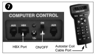
7. Slide the computer control panel power switch to OFF, if necessary. Remove the Autostar handbox and the Autostar interface cable from the packing materials. Plug one end into the HBX port of the computer control panel and plug the other end into the Coil Cable port on the Autostar handbox.
