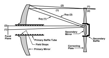
In the Schmidt-Cassegrain design of the Meade LX90, light enters from the right, passes through a thin lens with 2-sided aspheric correction ("correcting plate"), proceeds to a spherical primary mirror, and then to a convex secondary mirror. The convex secondary mirror multiplies the effective focal length of the primary mirror and results in a focus at the focal plane, with light passing through a central perforation in the primary mirror.
