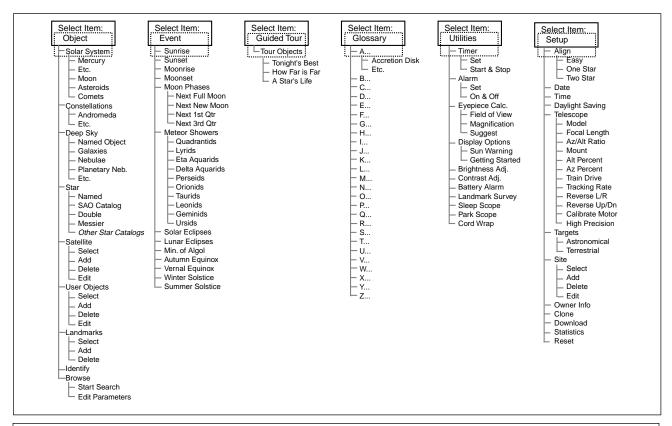
Figure 12: The Complete Autostar Menu Structure.
