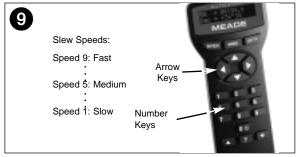
9. Press the key prompted by Autostar to accept the Sun warning. You can now use the Arrow keys to slew (move) the telescope up, down, right, or left. To change the telescope's slew speed, press the Number keys. "9" is the fastest speed and "1" is slowest speed. See page 16 for more details.
