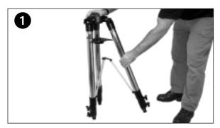
Remove the field tripod from the shipping carton. Stand the tripod vertically with the tripod feet down and with the tripod still fully collapsed. Grasp two of the tripod legs and, with the full weight of the tripod on the third leg, gently pull the legs apart to a fully open position.
