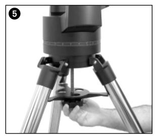
5. Take the LX90 from its packaging and place the entire telescope onto the top of the tripod head, inserting the threaded rod into the central hole in the bottom of the drive base of the telescope. Tighten the tension knob (see above figure) to a firm feel only; firm tightening of the tension knob is sufficient to result in rigid positioning of the tripod legs.
