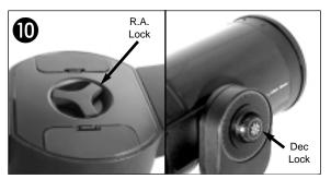
Tighten, to a firm feel only, the Dec and R.A. locks (6 and 9, Fig. 1). See page 7 for more information. Remove the dust cover from the end of the telescope tube.
