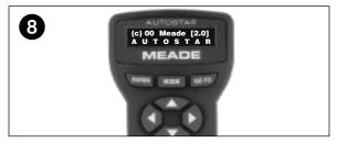
Flip the Power Switch on the computer control panel to the ON position. The copyright message lights on Autostar's LCD display.
