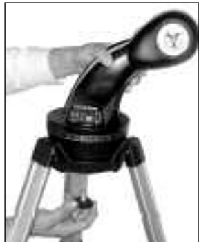
Fig. 5: Attach the mounting arm to the tripod base.
