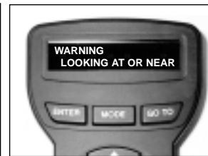
**Fig. 2:** Sun Warning on the Autostar LCD display.
